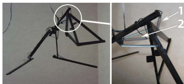
FIG. 7: The pair of active antagonistic wing-muscles.
